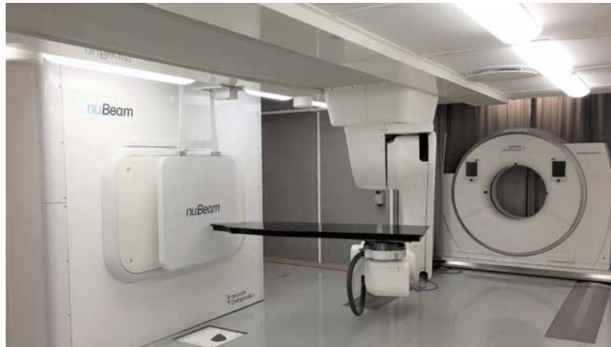
The new BNCT treatment room at the Helsinki University Hospital CCC, showing the beam-shaping assembly (left), robotic couch (centre) and in-room CT scanner (right). Courtesy: Neutron Therapeutics.
